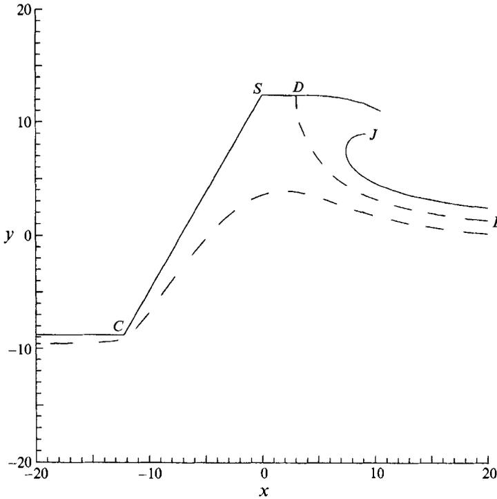
FIGURE 3. As figure 2 but for  $F_a = 1.68$ . The dashed lines represent the dividing streamline  $\psi = 0$ , which ends on the upper free surface, and the streamline  $\psi = 1$ .
