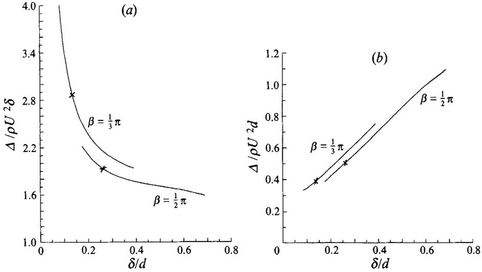
FIGURE 10. (a) Plot of the drag coefficient (see (3.8)) versus  $\delta/d$  for a vertical bow and  $\beta = \frac{1}{3}\pi$ ; (b) plot of the drag coefficient defined as  $\Delta/\rho U^2 d$ . The crosses indicate the transition for the location of the stagnation point  $D$ . For points on the left of the crosses,  $D$  is on the upper free surface. For points on the right of the crosses,  $D$  is on the bow.
