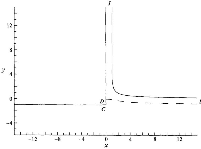
FIGURE 11. Computed solution without gravity for a vertical wall. The dashed line is the dividing streamline.
