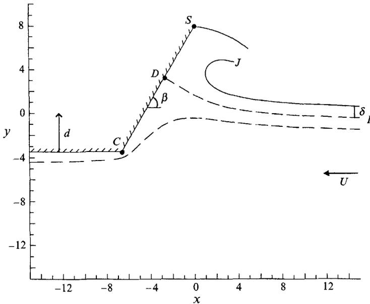
FIGURE 2. Sketch of a bow flow with spray. This is a computed solution for  $\beta = \frac{1}{3}\pi$  and  $F_a = 2.14$ . Five points have been selected on the boundaries. The dashed lines represent the dividing streamline  $\psi = 0$ , which terminates on the bow, and the streamline  $\psi = 1$ .
