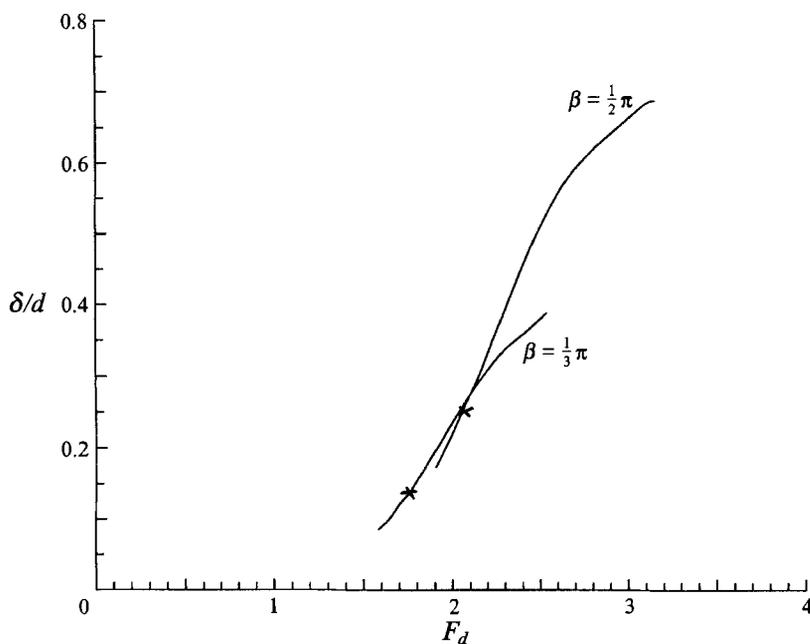
FIGURE 9. Plot of  $\delta/d$  versus  $F_a$  for a vertical bow and for  $\beta = \frac{1}{3}\pi$ . The crosses indicate the transition for the location of the stagnation point  $D$ . For points on the left of the crosses,  $D$  is on the upper free surface. For points on the right of the crosses,  $D$  is on the bow.
