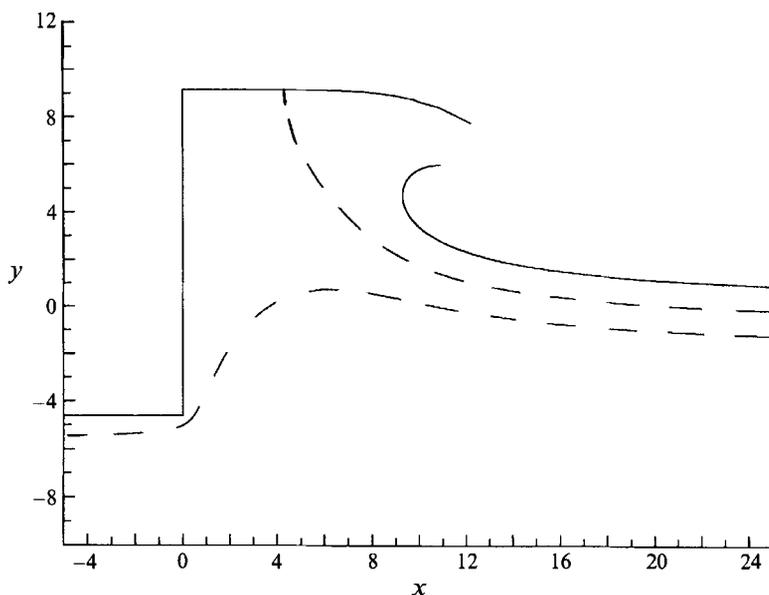
FIGURE 8. Computed solution with  $\gamma = \frac{2}{3}\pi$ . The resulting values are  $t_c = 0.548$ ,  $F_\delta = 4.28$ ,  $F_a = 1.99$ . The dividing streamline  $\psi = 0$  and the streamline  $\psi = 1$  are shown.
