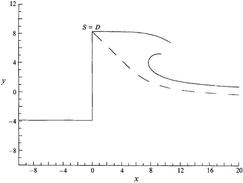
FIGURE 6. Computed solution with  $t_a = -1$ . The resulting values are  $t_c = 0.587$ ,  $F_\delta = 4.07$ ,  $F_a = 2.07$ . The dividing streamline  $\psi = 0$  is shown.
