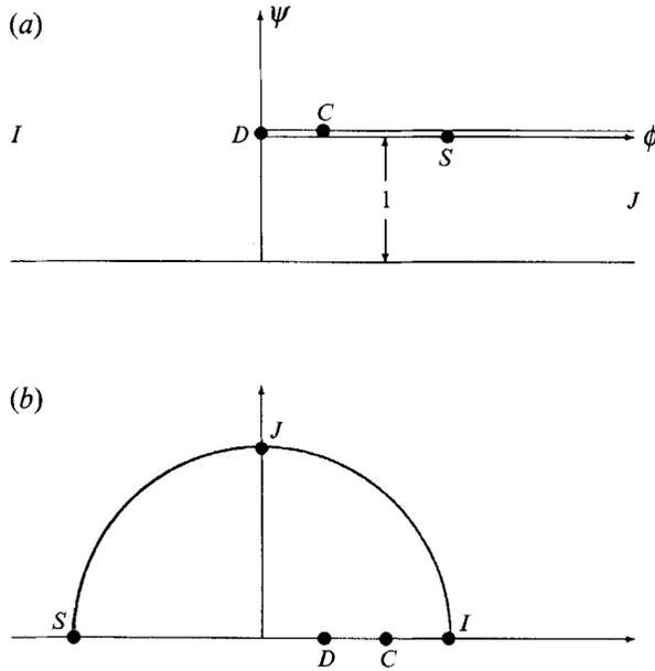
FIGURE 4. Flow domain in: (a) the plane of the complex potential  $f$ , (b) the intermediate  $t$ -plane. This case corresponds to bow flows where the dividing streamline ends along the bow. The images of the five selected points of figure 2 are shown.
