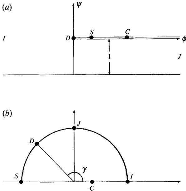
FIGURE 7. Flow domain in: (a) the plane of the complex potential  $f$ , (b) the intermediate  $z$ -plane. This case corresponds to bow flows where the dividing streamline ends on the upper free surface. The images of the five selected points of figure 3 are shown.
