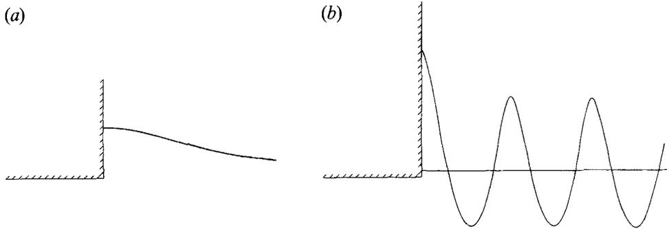
FIGURE 1. (a) Sketch of a bow flow with the free surface rising smoothly to a stagnation point on the bow. (b) Sketch of a bow flow with waves.
