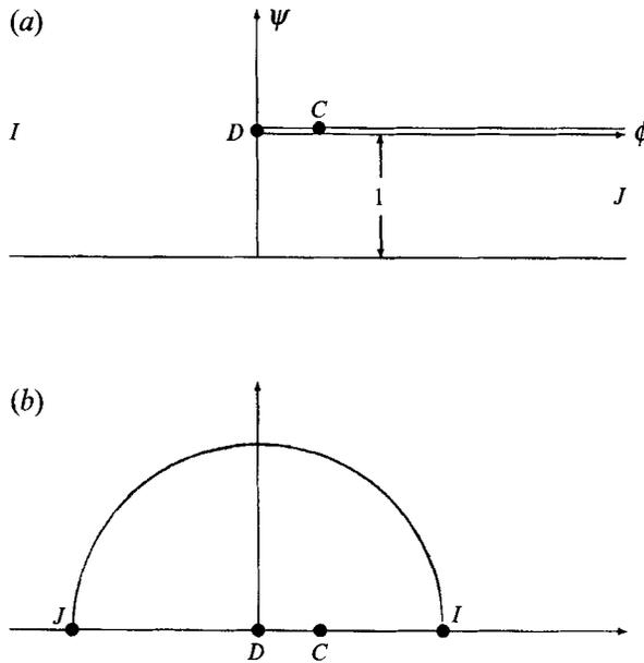
FIGURE 12. Flow domain in: (a) the plane of the complex potential  $f$ , (b) the intermediate  $t$ -plane. This case corresponds to flows without gravity. The images of the four selected points of figure 11 are shown.
