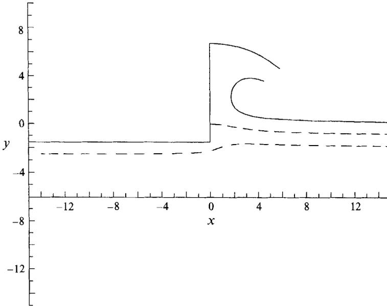
FIGURE 5. Computed solution with  $t_d = 0.935$ . The resulting values are  $t_c = 0.971$ ,  $F_\delta = 3.66$ ,  $F_d = 2.95$ . The dividing streamline  $\psi = 0$  and the streamline  $\psi = 1$  are shown.
